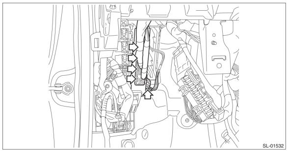
(2) Release the lock, and remove the data link connector bracket from the bracket.
